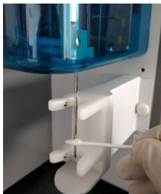
Figure 85. Wipe the Outer Surface of the Sample Injection Probe
