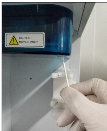
Figure 88. Wipe the SIP Cleaning Apparatus' Lower Surface
