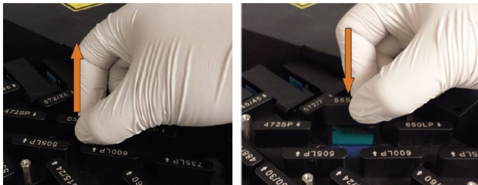
Figure 33. Remove the Old Filter and Insert the New Filter
