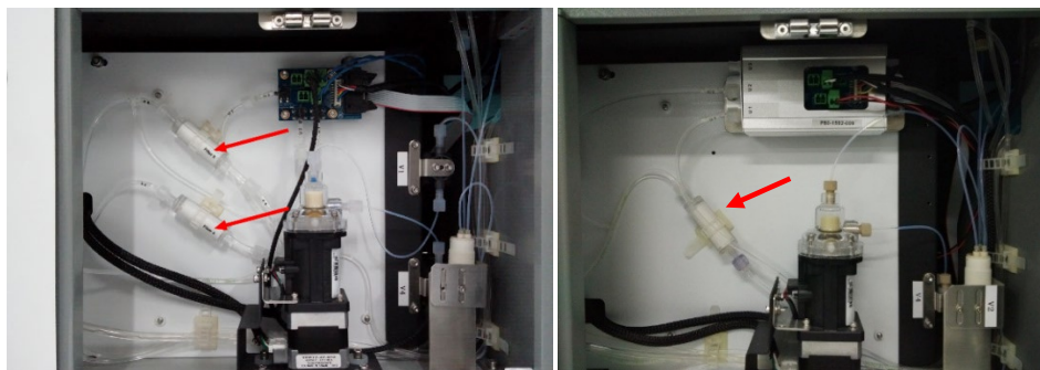
Figure 100. Location of Sheath Fluid In-line Filter in NovoCyte V1 Fluidics System (Left Figure) and NovoCyte V2 Fluidics System (Right Figure)
